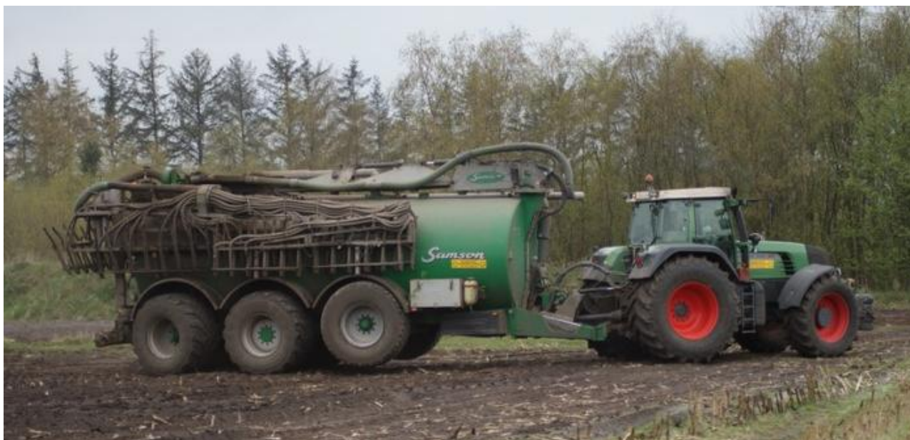
Picture 1: Typical machinery for transporting and spreading slurry, here configured with band laying system with a 24 metres wide boom.
